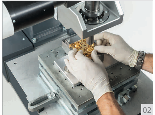
02 The torsional welding process developed and patented by TELSONIC greatly reduces the unwanted vibration input into the welded object.
