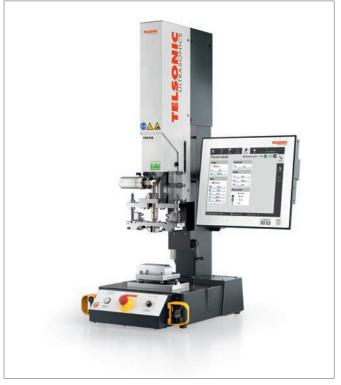
The application was welded using the torsional SONIQTWIST technology. The ultrasonic welding components were integrated into a special-purpose system.
