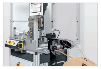
The application was realized on the MPX-RT ultrasonic welding system with an automatic feeder.
