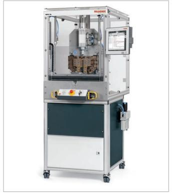
The application was realized on the MPX-GL ultrasonic welding system with automatic insulation crimping.
