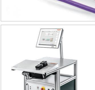
The applications were realized on Telso®Splice TS3 wire splicing systems.
